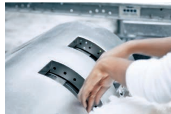
Top: Color measurement of the USTER® HVI 1000 utilizing the patented XENON FLASH
