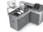
USTER® HVI 900 A Third generation of fiber length, fiber uniformity and short-fiber system
